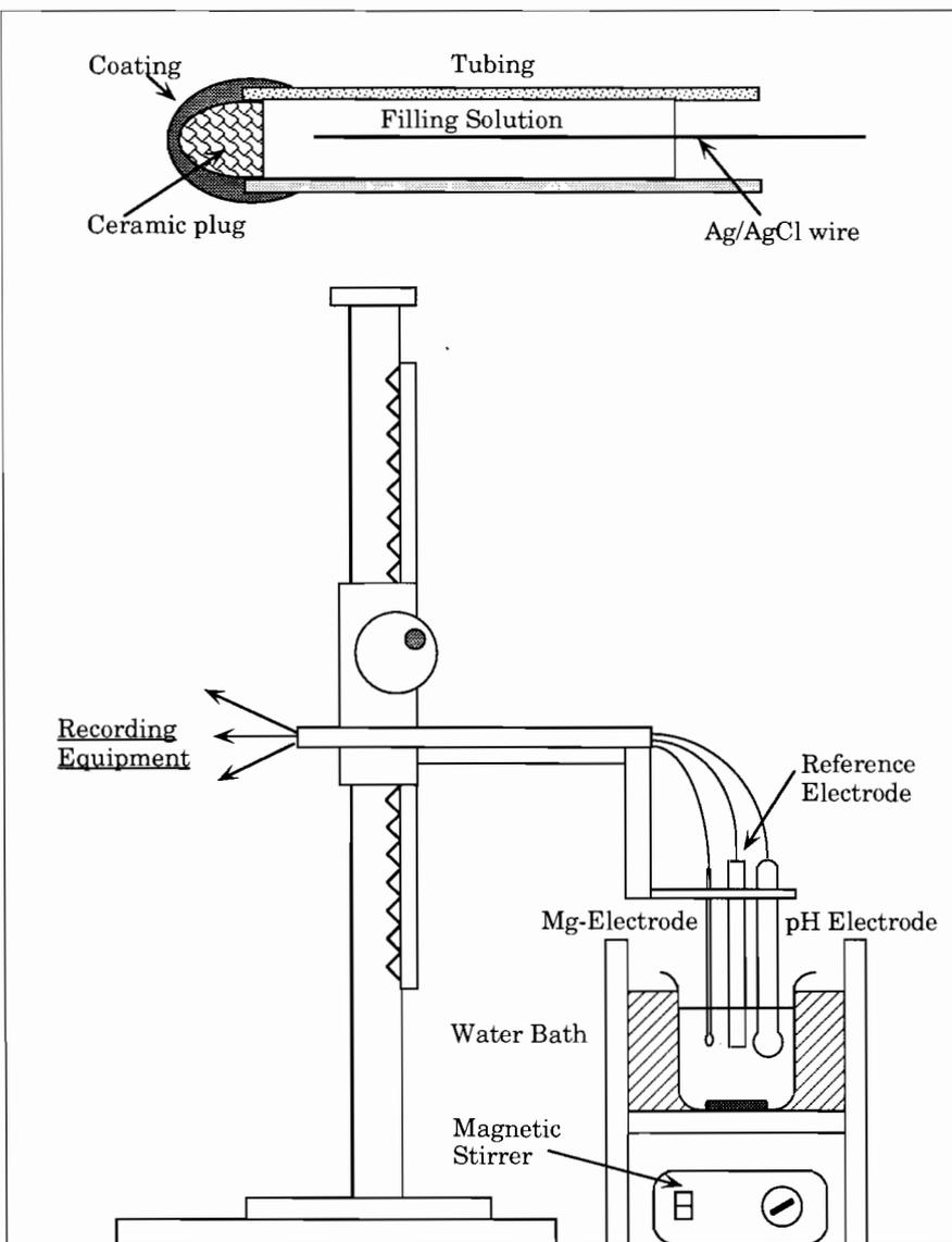
Fig. 1: Diagram of the experimental set-up used to either calibrate the electrodes or to measure apparent binding constants. All measurements were carried out at the same temperature and pH and solutions were pre-warmed to the desired temperature. A diagram of the electrode is shown at the top of the Fig.
