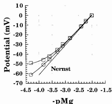
Fig. 2: Typical electrode calibration at 37 °C, circles immediately upon use and eight days later, squares. Both curves have been fitted by the modified *Nicolsky-Eisenman* equation. Coefficients of correlation,  $r$  were 0.9999 and 0.9994 respectively.
